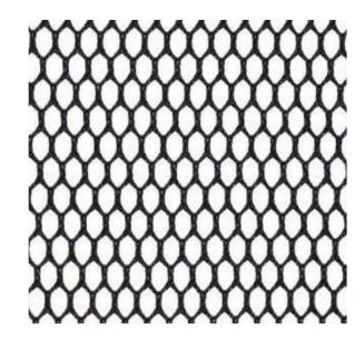
DNR25BK FR is knotless flame retardant netting with a 1/4 inch mesh. The polyester Raschel monofilament fiber is highly resistant to abrasion, and is resistant to moisture and most chemicals. ASTM F2375 Class 1 compliant.
